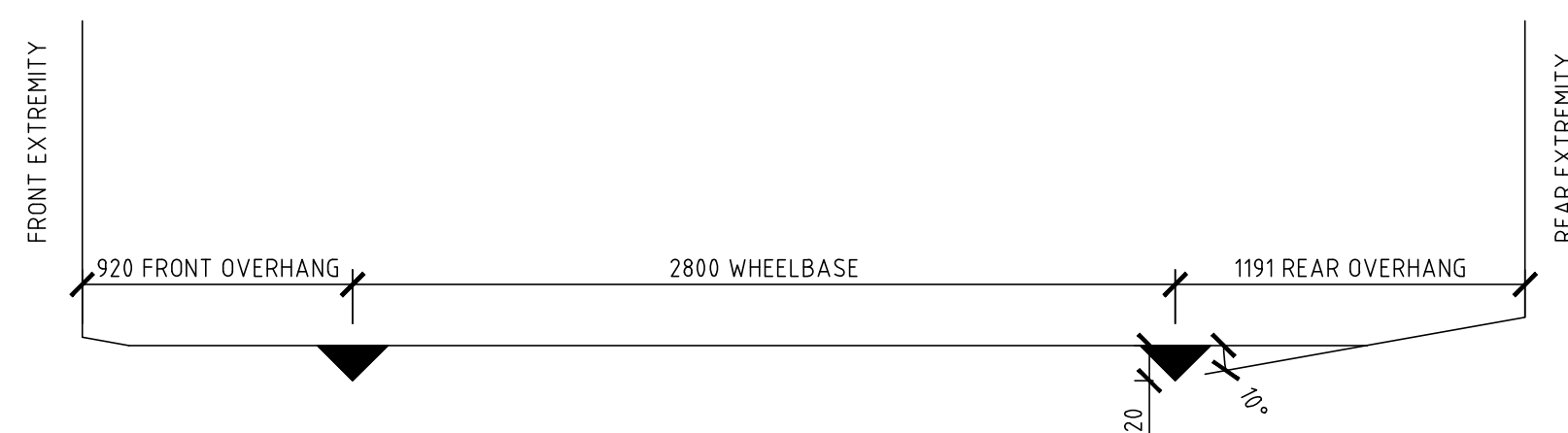
GROUND CLEARANCE TEMPLATES FOR B85 VEHICLE
